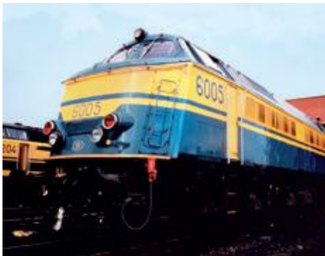
Locomotiva Diesel Electrica 6005, SNCB-NMBS 6DZC, 1350KW(1800CP)
