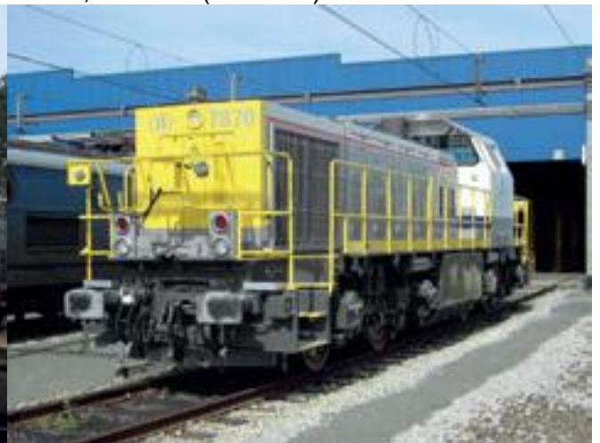
Locomotiva Diesel Hidraulica HLD77, SNCB-NMBS 6DZC,1150KW(1560CP)
