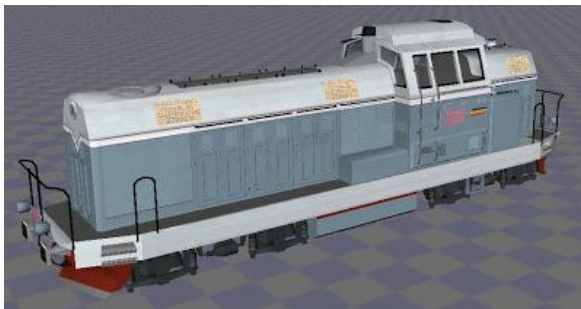
REMOTORIZARE LOCOMOTIVA LDE1250 CU MOTOR ABC 6DZC-1000-176 1405KW(1910HP)/1000RPM
