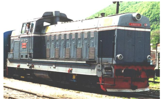
REMOTORIZARE LOCOMOTIVA LDE2100 CU MOTOR ABC 8DZC-1000-176 1875KW(2545HP)/1000RPM
