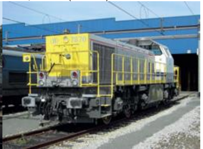
Diesel Hidraulic locomotive HLD77, SNCB-NMBS 6DZC,1150KW(1560HP)
