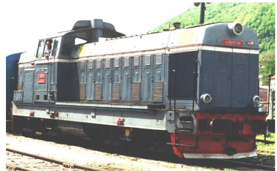
REFURBISHMENT LOCOMOTIVE LDE2100 WITH ABC ENGINE 8DZC-1000-176 1875KW(2545HP)/1000RPM
