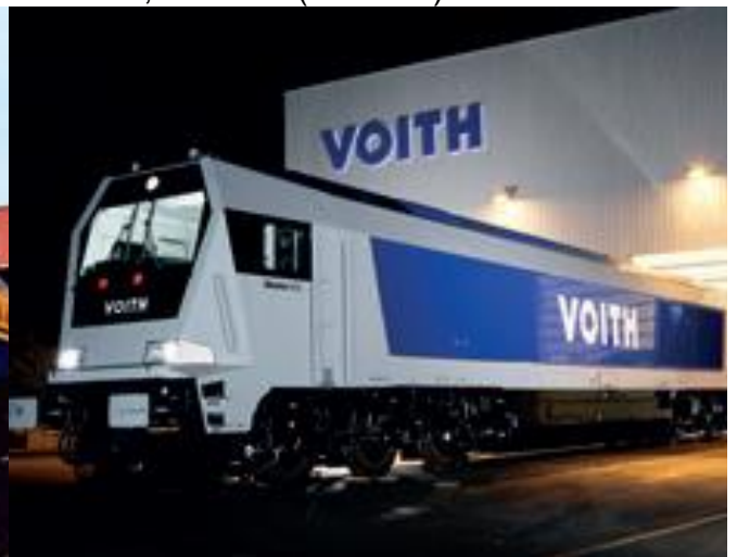
Diesel Hydraulic locomotive VOITH MAXIMA 40cc (the most powerfull hydraulic mono-engine locomotive) 16VDZC, 3600KW(4900HP)
