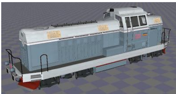
REFURBISHMENT LOCOMOTIVE LDE1250 WITH ABC ENGINE 6DZC-1000-176 1405KW(1910HP)/1000RPM
