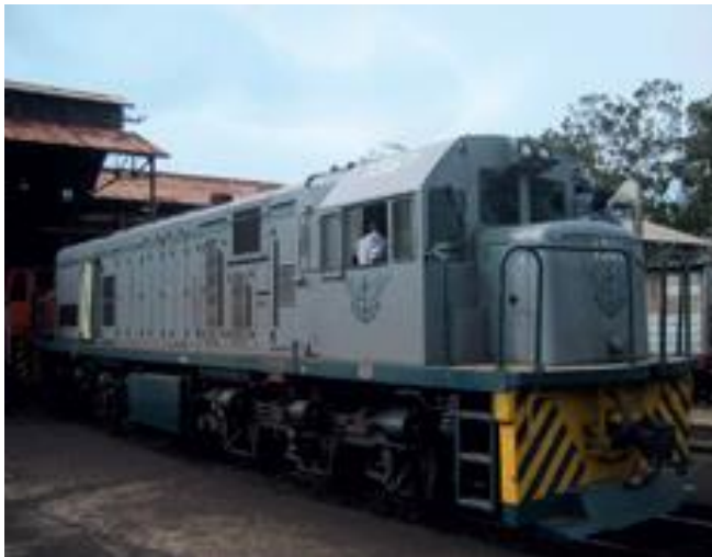
Diesel Electrical locomotive U15, ONATRA 6DZC, 1150KW(1560HP)
