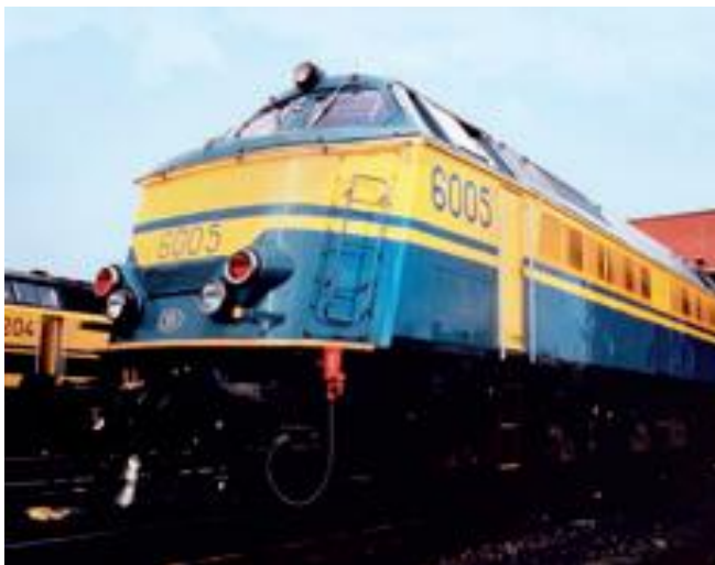
Diesel Electric locomotive 6005, SNCB-NMBS 6DZC, 1350KW(1800HP)
